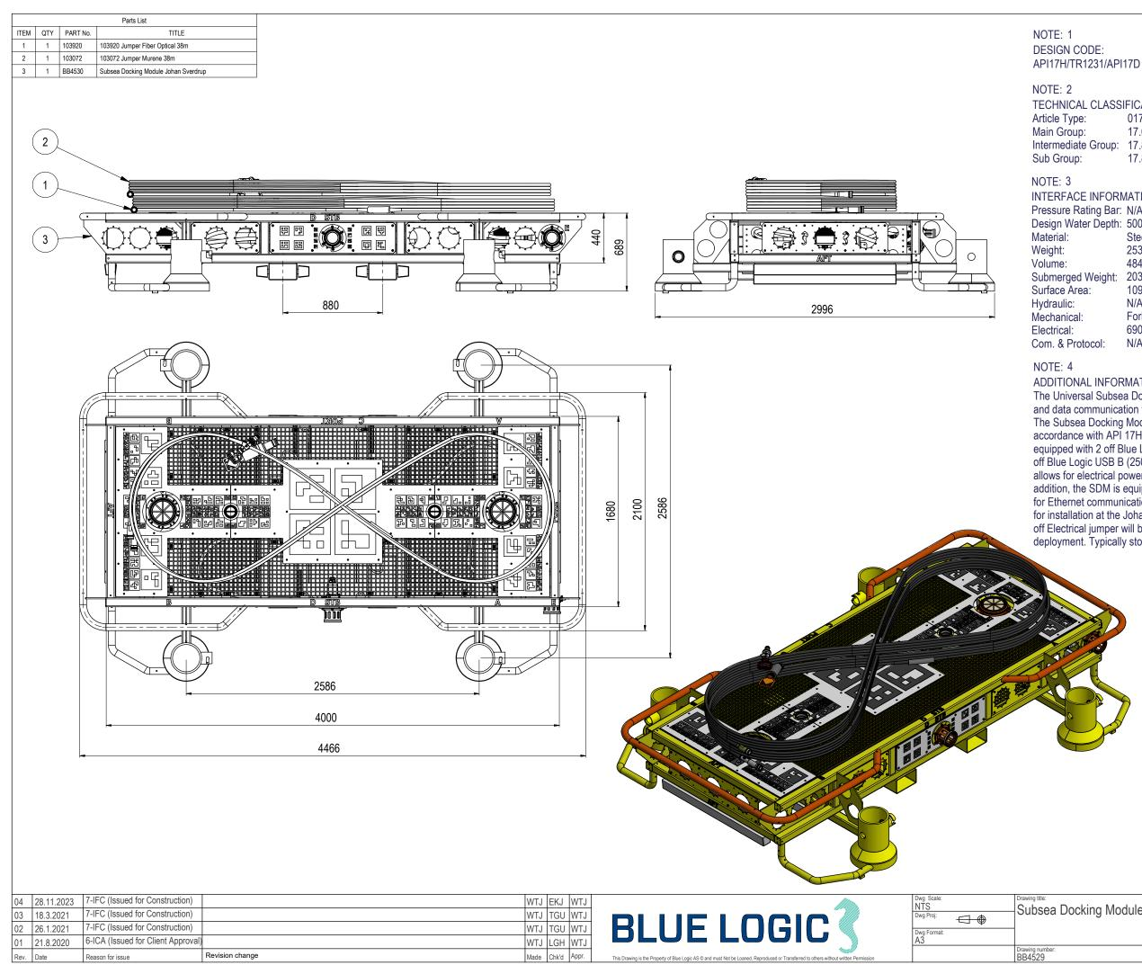
TECHNICAL CLASSIFICATION: 017-Drone Charging 17.01. UID Charge Station Intermediate Group: 17.80.03. Docking Module 17.80.384.01. Steel Structure INTERFACE INFORMATION: Pressure Rating Bar: N/A Design Water Depth: 500m Steel 2535,2 kg 484,26 dm^3
