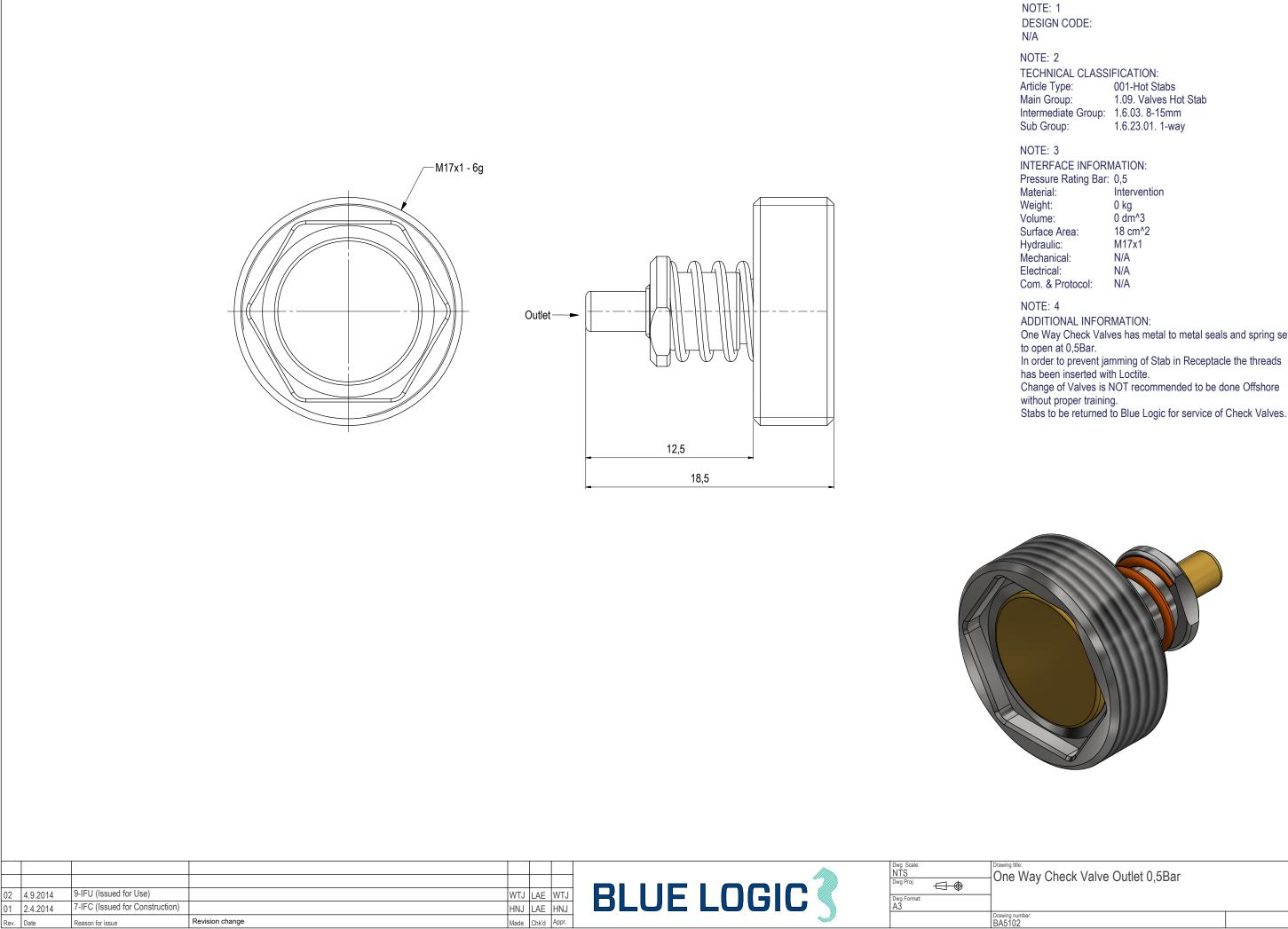
One Way Check Valves has metal to metal seals and spring set In order to prevent jamming of Stab in Receptacle the threads Change of Valves is NOT recommended to be done Offshore
