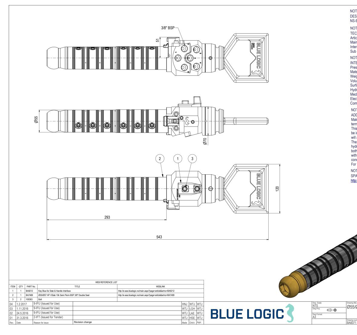
NOTE: 1 DESIGN CODE: NS-EN 13445:2009 / ISO 13628-8 NOTE: 2 **TECHNICAL CLASSIFICATION:** Article Type: 003-Valve Stabs Main Group: 3.07. Dual Bore-Valvestab Intermediate Group: 3.42.1. Stab Sub Group: 3.42.102.6. Hexa NOTE: 3 INTERFACE INFORMATION: Pressure Rating Bar: 690 Material: Semi Permanent 9,3 kg Weight: Volume: 1,26 dm^3 3704 cm^2 Surface Area: 3/8" BSP Hydraulic: D-Handle Mechanical: N/A Electrical: N/A Com. & Protocol:
