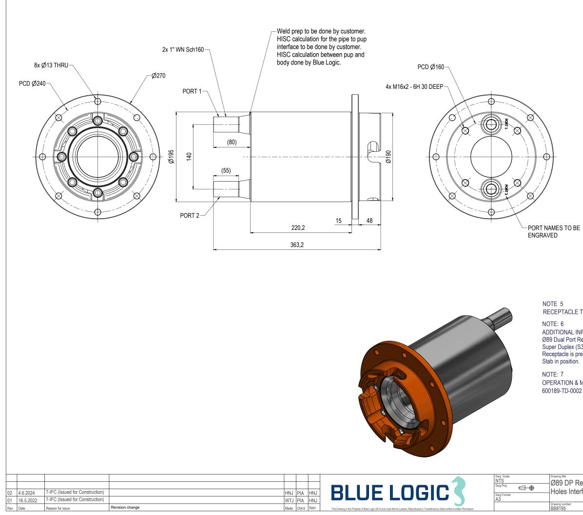
NOTE: 1 DESIGN CODE: API 17H Type 3 NOTE: 2 TECHNICAL CLASSIFICATION: Article Type: 001-Hot Stabs Main Group: 1.10. Ø89 Hot Stab Intermediate Group: 1.89.02. Receptacle Sub Group: 1.89.423.02. Dual NOTE: 3 INTERFACE INFORMATION: Pressure Rating Bar: 690 Design Water Depth: N/A Material: Long-term 48,9 kg Weight in Air: 6,23 dm^3 Volume: Submerged Weight: 42,52 kg 5085 cm^2 Surface Area: 1" WN Sch 160 Hydraulic: Mechanical: N/A N/A Electrical: Com. & Protocol: N/A
