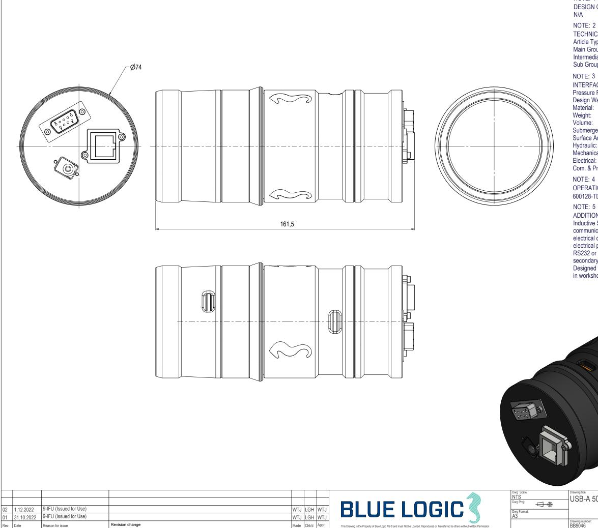
NOTE: 1 DESIGN CODE: NOTE: 2 **TECHNICAL CLASSIFICATION:** Article Type: 006-El. Connectors Main Group:6.01. Subsea USBIntermediate Group:6.28.01. 0-60W Subsea USB Sub Group: 6.28.95.01. Male Connector NOTE: 3 INTERFACE INFORMATION: Pressure Rating Bar: N/A Design Water Depth: N/A Material: N/A 0,5 kg 0,37 dm^3 Submerged Weight: 0,15 kg Surface Area: 2244 cm^2 Hydraulic: N/A Mechanical: N/A Electrical: N/A Com. & Protocol: N/A
